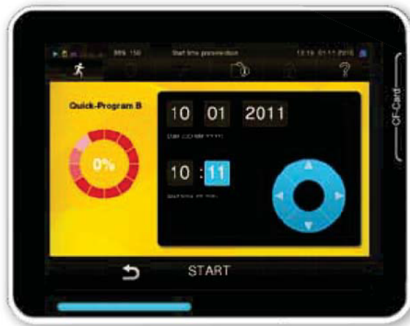
Time pre-selection for automatic autoclave start
